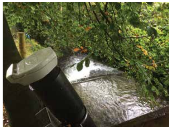
Stilling well with DTT Instrumentation. Stream channel, bridge and V notched weir.
