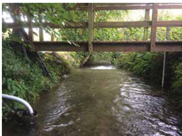
Stilling well with DTT Instrumentation. Stream channel, bridge and V notched weir.
