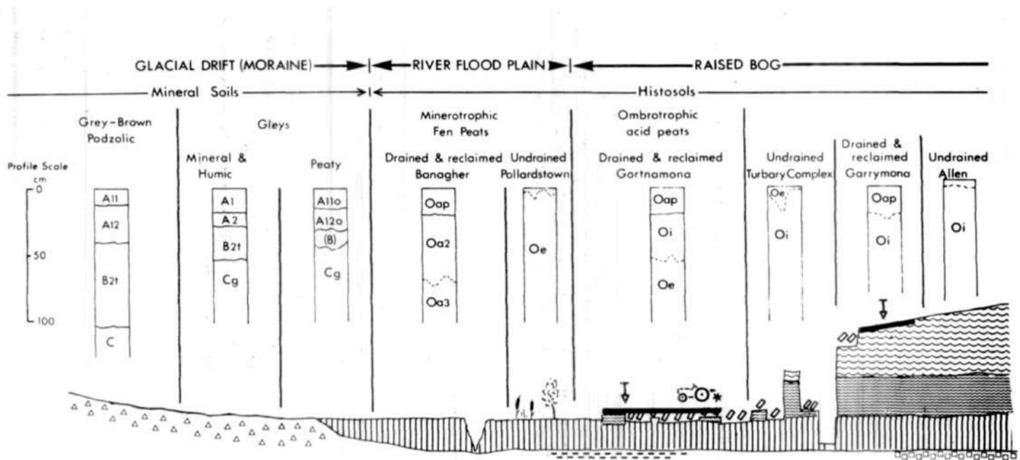
Figure 6: Schematic cross section of typical landscape with organic soils in the Irish midlands
