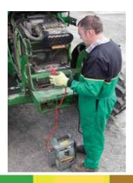
When using jump leads connect the negative lead to a good earth point at least 500mm from the discharged battery.
