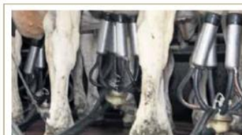
The wash programme needs to include detergent to clean milk residues and acid to clean mineral deposits from water.
