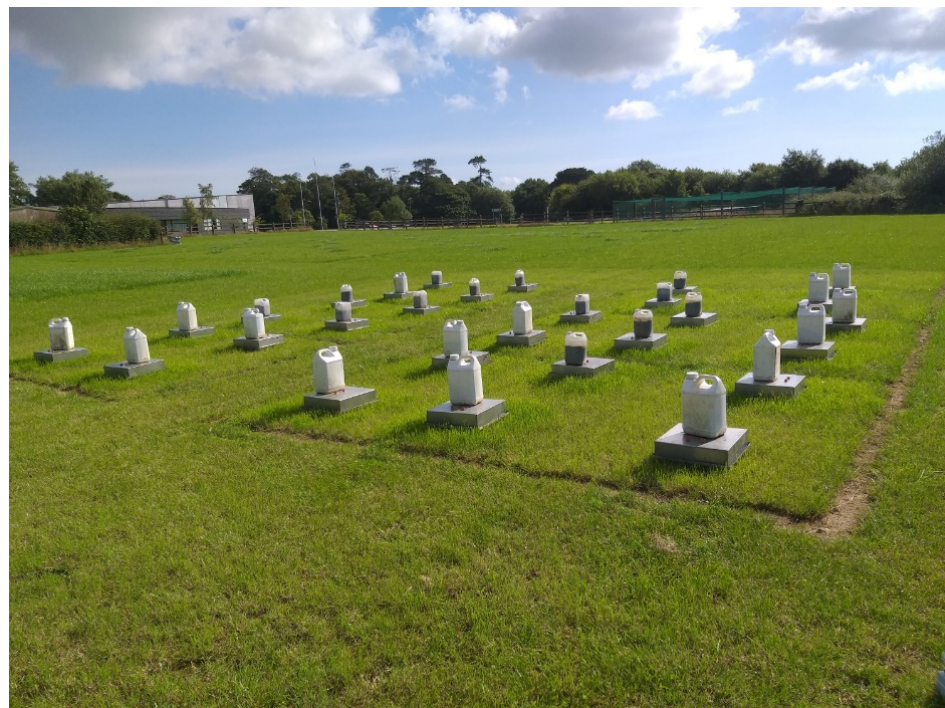
Figure 1. Photograph of experimental field (grassland) at Johnstown Castle research site during gas sampling from static chambers with the square collars inserted into the soil and lead covers closed with ballast weights placed on top.
