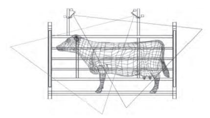
Figure 1. Camera positioning of the automated BCS system
