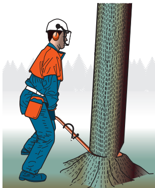
Figure 3: Use of breaking bar
