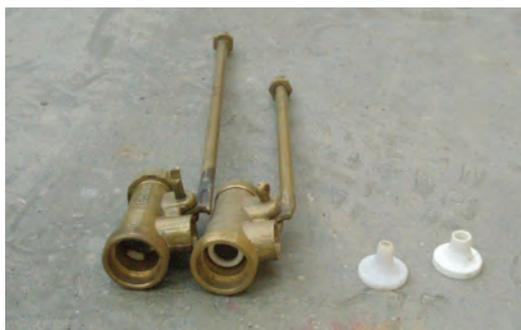
**Photo 2.** Two standard  $\frac{1}{2}$  inch ballcocks, one showing a shorter float arm. High and medium pressure jets can be used with this type of ballcock.
