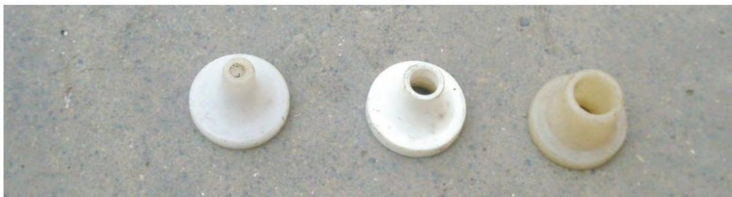
**Photo 1.** The high-pressure jet has the smallest hole and the low-pressure jet the biggest.
