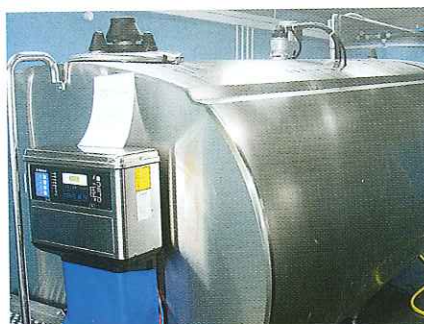
Milk can be cooled by a tank that uses direct expansion or by water delivered from an ice bank positioned at the base of the bulk tank.
