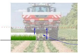
Check operators manual, ensure tractor and spreader are compatible. Fit front weights as necessary. Check tractor controls
