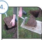
Carefully lever out the sample block on the spade and place on a plastic sheet or tray.
