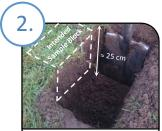
Dig a hole, wider and deeper than an intended sample block. Do not stand on or lean the spade against the sample block.
