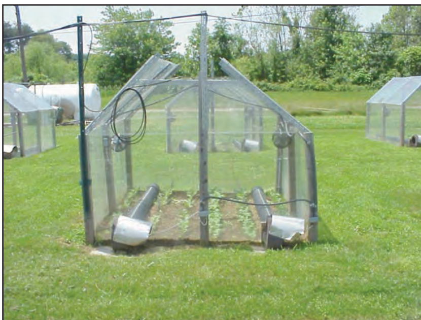
Figure 2. A typical open top chamber. (Image courtesy ASDA, ARS)
