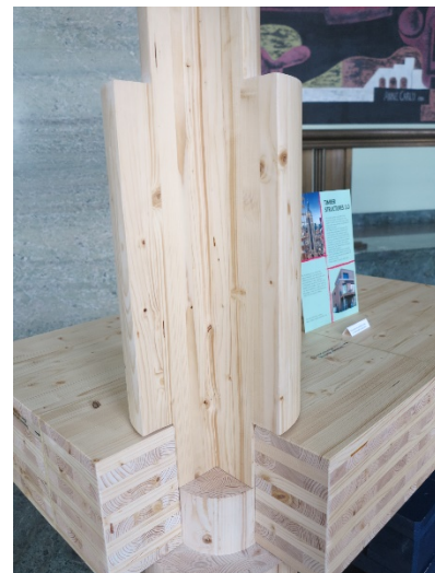
Plate 5: Cross-Laminated Timber, Source: DRIMA.ie
