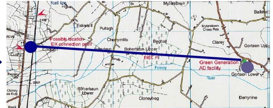
~ 5 km low pressure biogas pipeline
