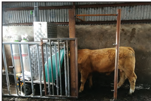
Figure 1. The first GreenFeed Emissions Monitoring System used to estimate enteric methane emissions at the ICBF Progeny Performance Test Centre in Tully (Co. Kildare).
