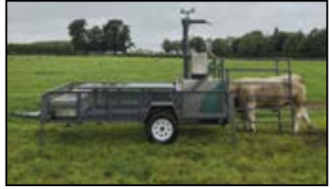
Figure 1. The GreenFeed Emissions Monitoring System used to estimate enteric methane emissions from grazing beef cattle in Teagasc Grange.
