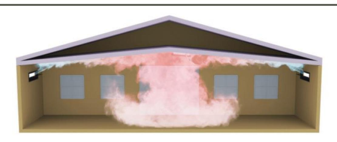
Proper Inlet System directs air along the ceiling to center of house before it drops to the floor level.
