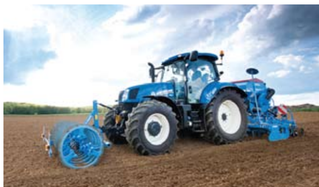
Cultivator/drill working on ploughed ground
