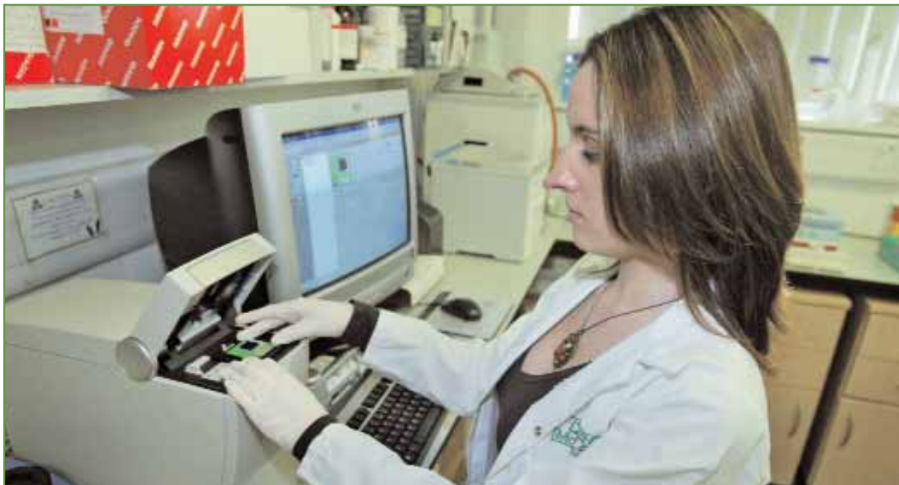
Nucleic acid analyser at Moorepark used to measure DNA quality. Pictured is Olivia McAuliffe, Research Officer in the Biotechnology Department.
