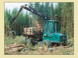
Crucial to the cost-effectiveness of a forwarder is the distance it has to travel to the collection point. The increased cost of forwarding may significantly affect thinning costs beyond an optimal extraction distance of 250-300 metres.
