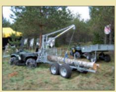
Quad with trailer and loading crane
