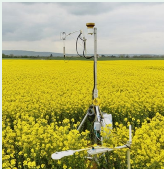
Carbon flux tower quantifying carbon fluxes in a rape field and the location of the National Agricultural Soil Carbon Observatory sites across Ireland.
