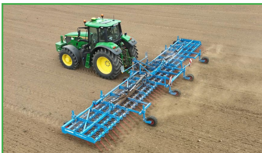
Mechanical weeding (Pre Emergence) with the LEMKEN Thulit on a participating farm
