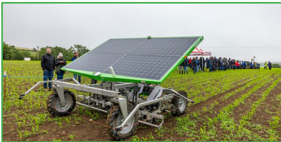
FarmDroid autonomous seeding and weeding system
