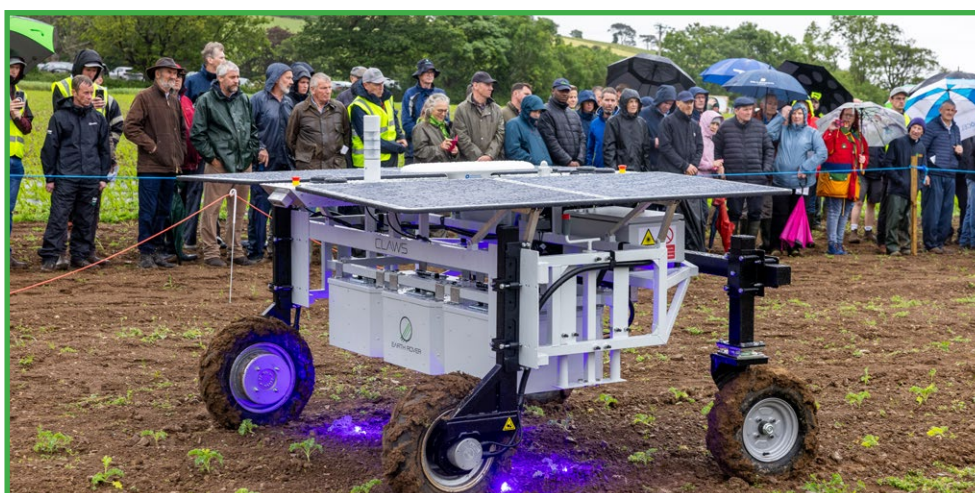
Earth Rover CLAWS laser weeding technology
