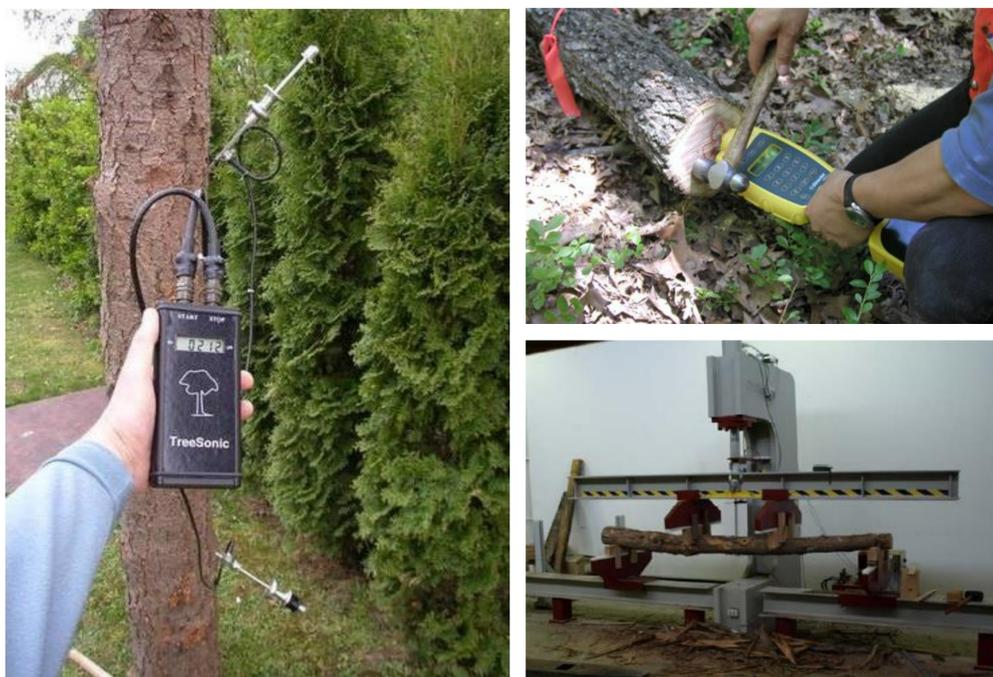
Fig. 2 : NDT measurements on standing trees(a), logs (b) and mechanical test (c)
