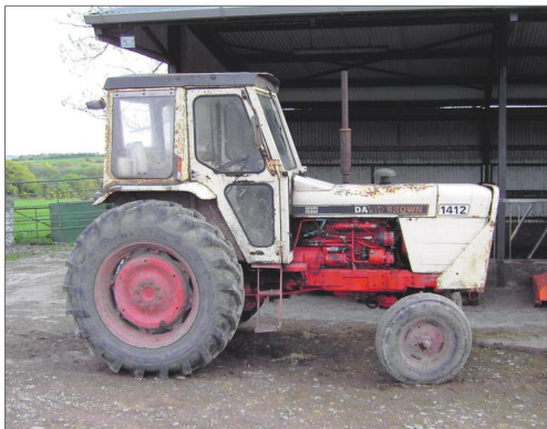
David Brown launched its Q cab in 1975 and later upgraded to the VQ cab in 1977, as shown here, with its widened doors for easier access.
