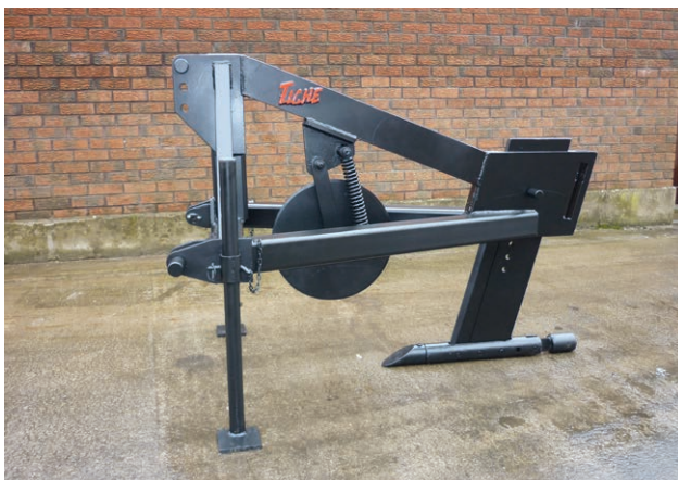
Figure 12. Mole plough showing cylindrical foot and expander
