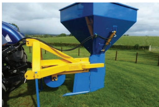
Figure 13. Gravel mole plough showing hopper
