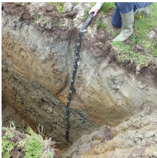
Figure 10. Test pit excavation
