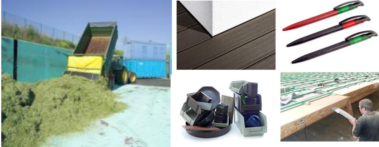
Products produced from grass: injection moulded products, terrace profiles, ballpoint-pen, insulation material (source: www.biowert.de )
