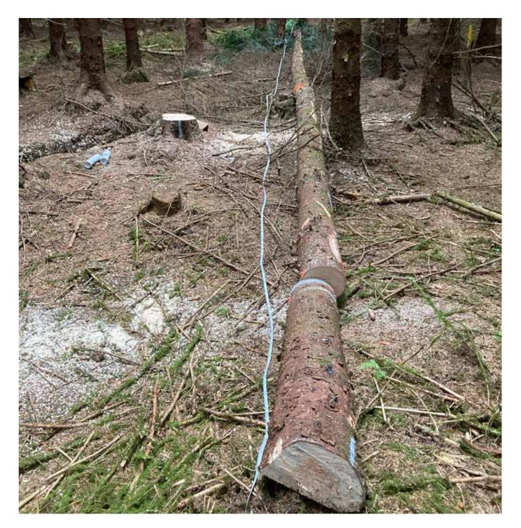
Figure 5: Felling and taking discs from sample Sitka spruce for tree ring analysis to study if drought conditions can be detected.
