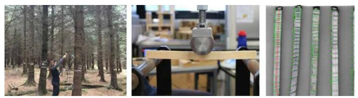
Figure 7: Testing timber quality of Sitka spruce families using a TreeSonic<sup>™</sup> (left) which measures time of flight between two probes and has been linked to bending strength of timber (middle photo) and ring width analysis using the WinDENDROM<sup>™</sup> system.
