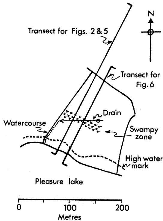
Fig. 3: A site plan showing seep zone, drain location and position of transects
