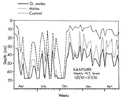
Fig. 7: Water level fluctuations at Kanturk
