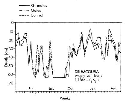
Fig. 3: Water level fluctuations at Drumcoura
