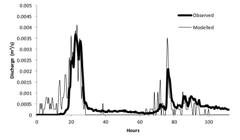
Figure 1. Comparison of tile drain discharge from modelled SEEP/W analysis and observed field measurements in System 1 during the calibration event (Event A)
