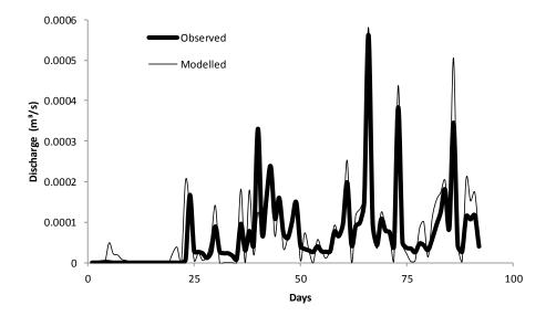
Figure 2. Comparison of daily tile drain discharge from modelled SEEP/W analysis and observed field measurements in System 1 during the validation event (Event B).
