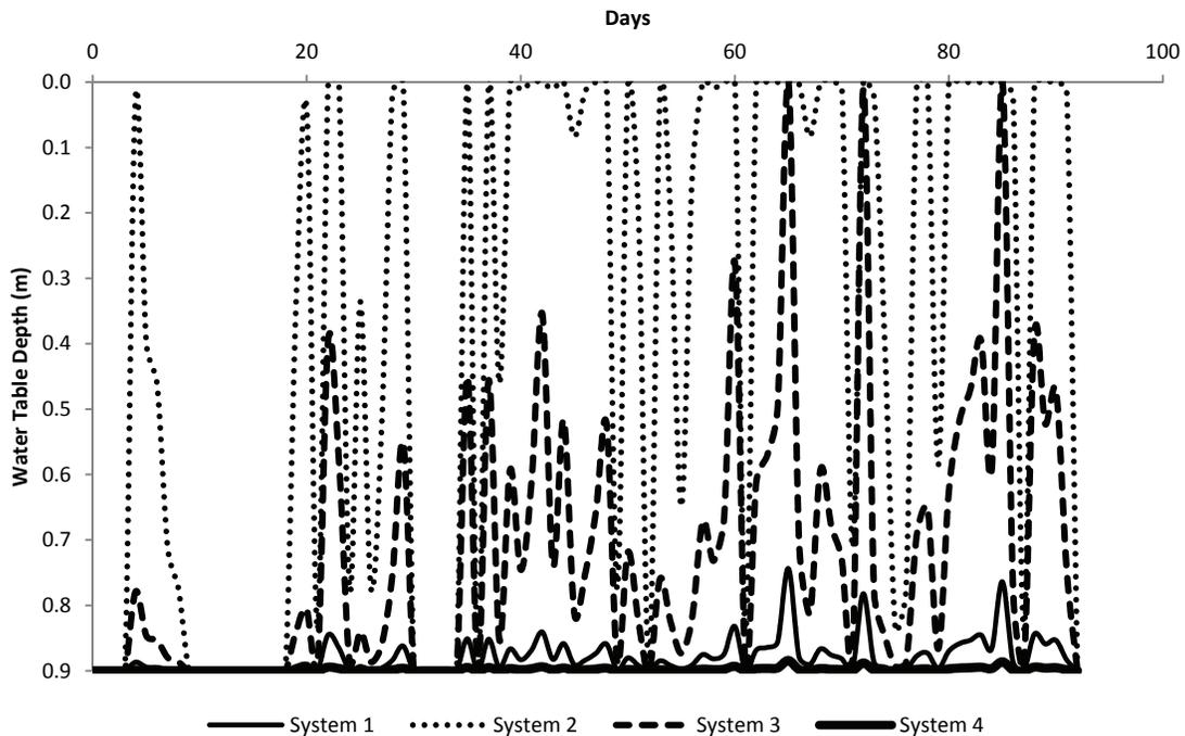
Figure 8. Modeled water table depth 7.5 m from tile drain center (mid-drain spacing) for systems 1 through 4 during event B.
