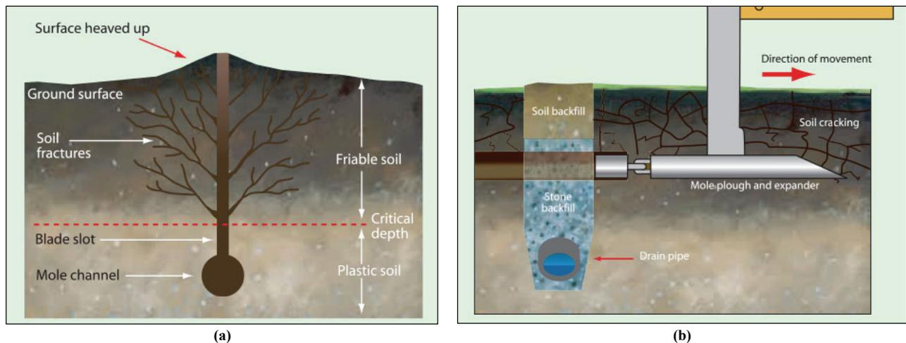
Figure 1. Cross-sections of (a) mole drain channel and (b) tile drain with stone aggregate backfill and intersecting mole drain.
