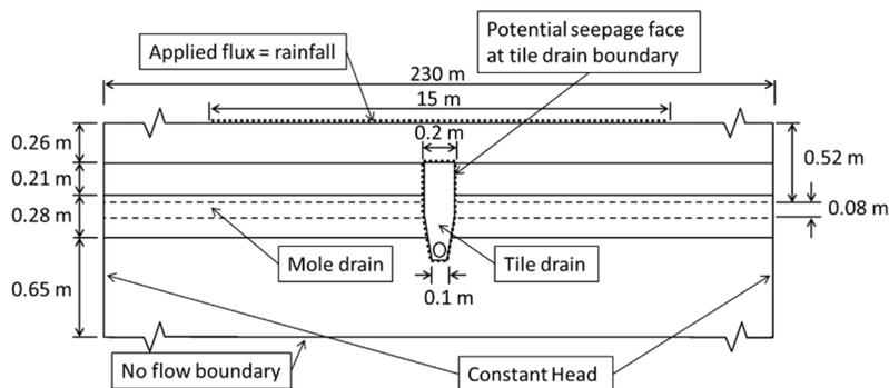
**Figure 2. Cross-section of modeled system showing system geometry and boundary conditions (not to scale).**
