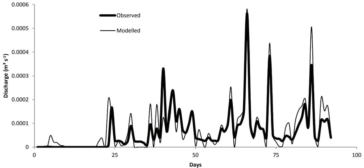
Figure 4. Daily tile drain discharge from SEEP/W analysis and observed field measurements in system 1 during event B (validation).
