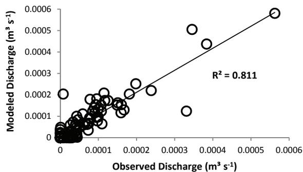
Figure 5. Modeled versus observed daily tile drain discharge ( $\text{m}^3 \text{s}^{-1}$ ) from system 1 during event B (validation).
