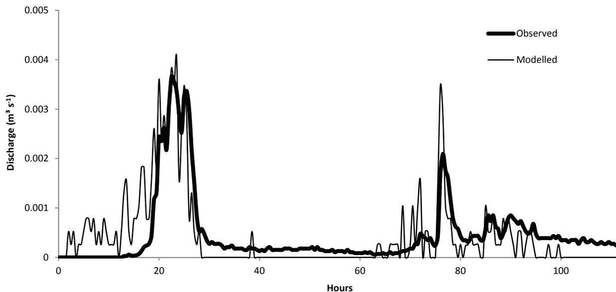
**Figure 3. Tile drain discharge from SEEP/W analysis and observed field measurements in system 1 during event A (calibration).**
