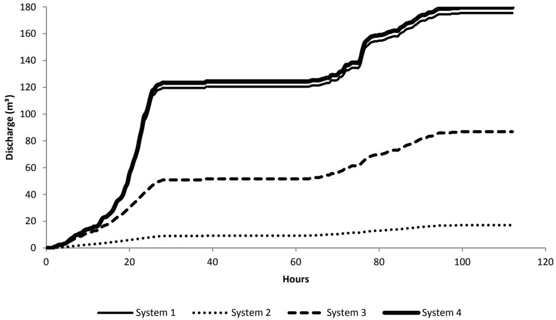
Figure 7. Modeled cumulative tile drain discharge during event A.
