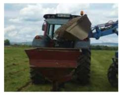
Fig. 3a. Gravel Mole plough showing hopper
