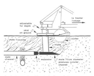
Fig. 4. Mole ploughing showing intersection with a piped collector drain
