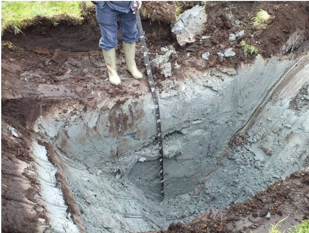
Test hole 2 at 3 metres deep
