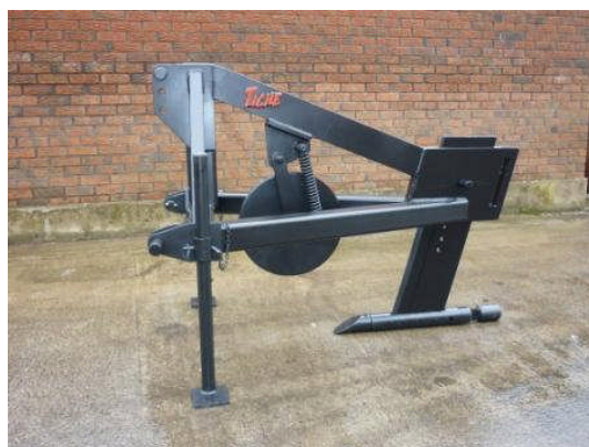
Fig. 2a .Mole plough showing cylindrical foot and expander, 2b. Cracking and channel formation
