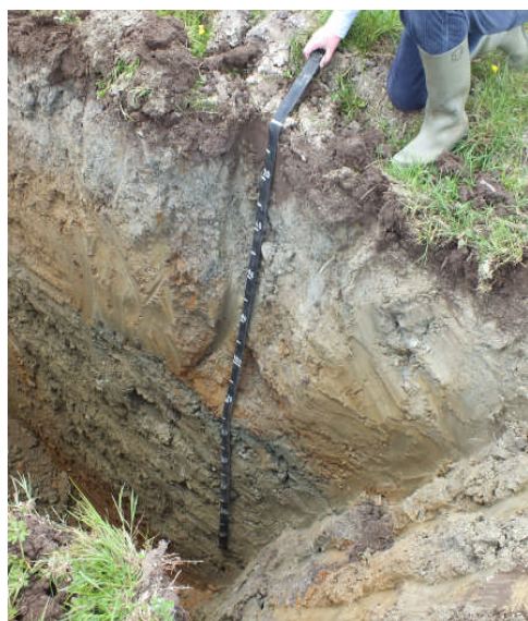
Fig. 1a .Test pit excavation
