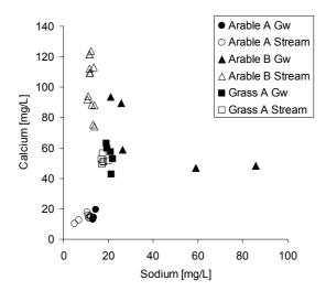
Fig. 2. Ca and Na concentrations in the stream (monthly samples) and near-stream groundwater (means of monthly samples) across a range of depths (2-50m) in each catchment.
