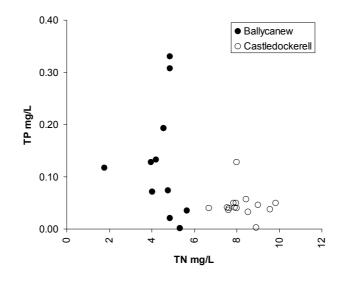
Fig. 1. Total phosphorus and total nitrogen concentrations in a series of preliminary validation water samples from outlets of the Castledockerell (predicted as highly susceptible to N transfer) and Ballycanew catchments (predicted as highly susceptible to P transfer).
