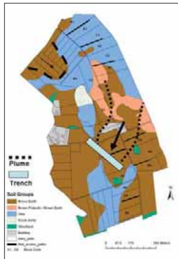
Contamination migration intercepted by denitrification trench.
