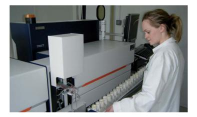
Teagasc, Moorepark, is currently researching the potential use of mid-infrared spectrometry technology to determine the energy balance status of cows at the time of milk recording.
