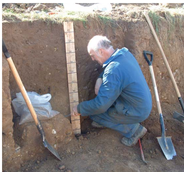
Ground-truthing: methods for mapping our soils must include traditional soil profile descriptions such as here at Kilmallock, Limerick.
