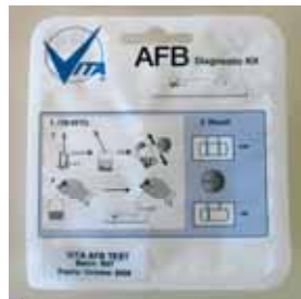
Plate 40: AFB kit (Vita® Europe Ltd.) which can be used for the detection of AFB in the field
