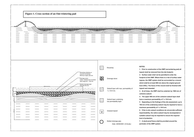
Figure 1 shows a typical cross section of a soil-lined OWP
