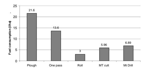
**Fig 2:** Estimated fuel consumption for different cultivation operations.
