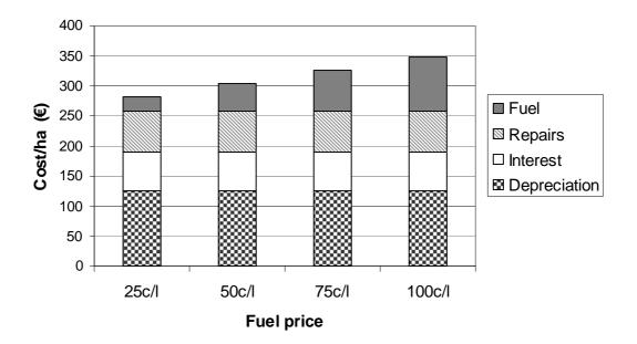
Fig 1: The increasing effect of fuel price on machinery cost elements
