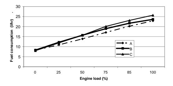
**Fig 6:** Tractor fuel consumption for newer and older tractor models at 80kW power output
