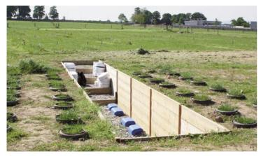
Lysimeters installed at Teagasc, Moorepark, to monitor nutrient leaching and  $N_2O$  emissions.
