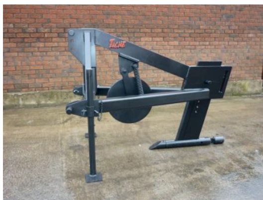
Fig. 2a .Mole plough showing cylindrical foot and expander, 2b. Cracking and channel formation
