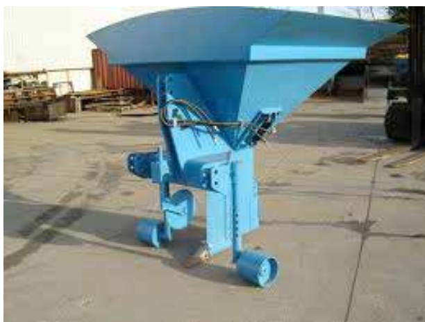
Figure 7. Gravel mole plough showing hopper
