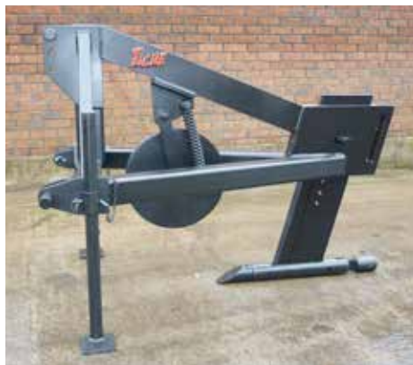
Figure 6: Mole plough showing foot and expander
