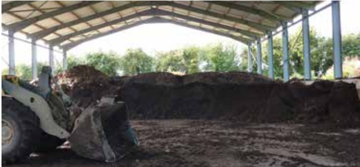
SMCs stored under cover and protected from rain had lower H 2 S emissions during compost disturbance.
