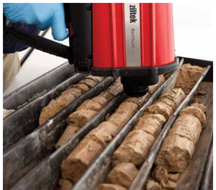
Photograph of RemScan, a hand-held instrument for the rapid measurement of total petroleum hydrocarbons (TPH) in soil. Images courtesy of RemScan manufacturer Ziltex. www.ziltex.com
