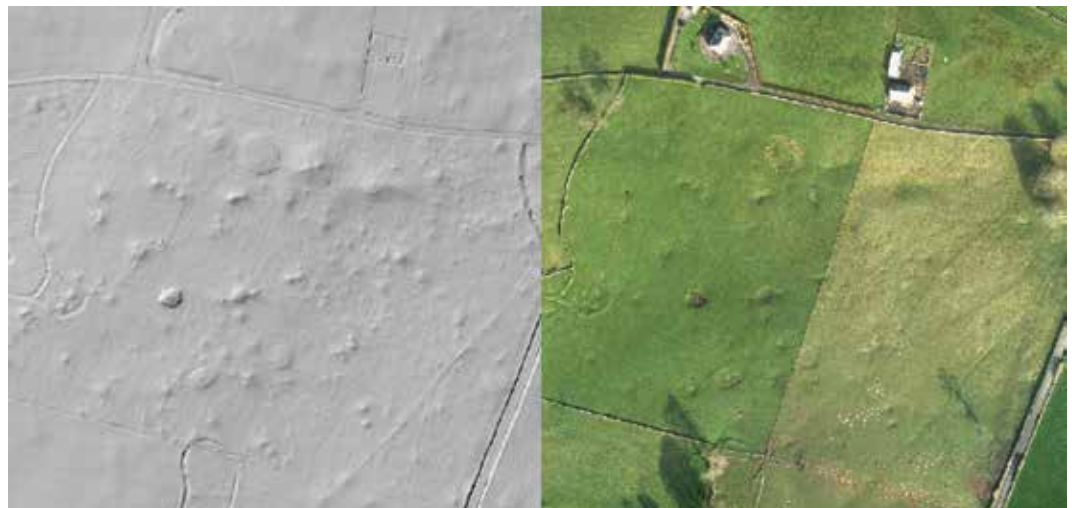
Figure 1. Right: ortho photo (geometrically corrected aerial photo). Left: LiDAR (light detection and ranging) image of a doline field in an agricultural karst spring zone of contribution. These images can be used to map surface karst features.
