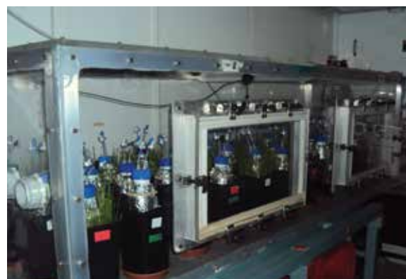
Steady-state isotope labelling chamber: ^{13}\text{C} -labelled \text{CO}_2 at ambient concentrations is passed through the chamber over the growth period of the plant. Use of stable isotopes allows for differentiation between photo-assimilated C and soil-derived C in total \text{CO}_2 efflux to quantitatively measure plant-C inputs and soil-C outputs.
