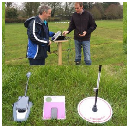
Figure 4. CONNECT Pervasive Nation IoT Low power wide area network platform deployment (top), optical, smart phone and plate meter sensing/measurement (bottom)
