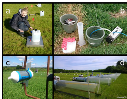
Figure 3. Overview of experimental methodology used; a) N 2 O sampling with the static chamber method, b) nitrate leaching sampling with lysimeters, c) NH 3 sampling with shuttle method (IHF), d) NH 3 sampling with windtunnels.
