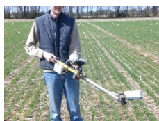
Figure 2. Optical sensing and hand held x-ray fluorescence testing
