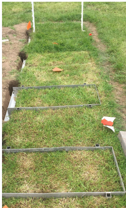
Figure 2: Micro-plot rainfall simulation study site – (top) Amsterdam drip-type rainfall simulator, (middle) Series of isolated grassland micro-plots and (bottom) Individual plot isolated by steel frame of dimension 0.9 m in length and 0.4 m in width with runoff collection channel.
