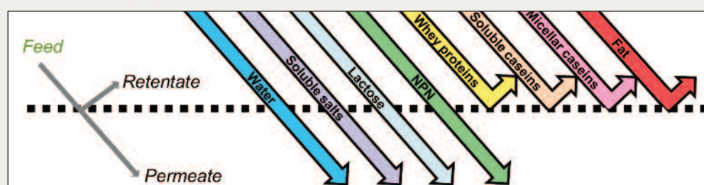
FIGURE 1: Partition of milk components by microfiltration (MF) and ultrafiltration (UF).
